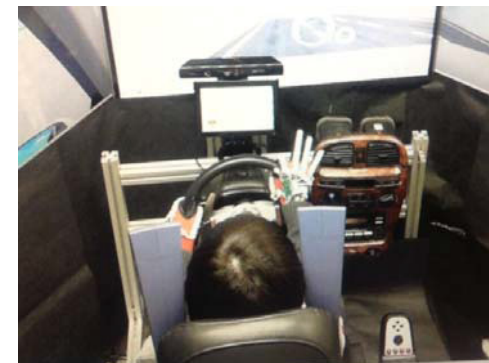
Figure 4: HUD-installed driving simulator.
