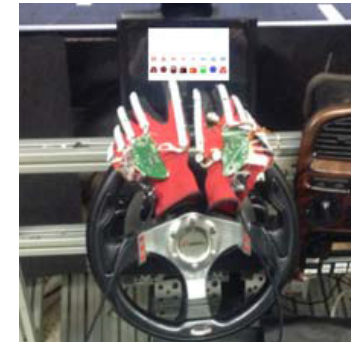
Figure 3: Essential Reality P5 Gaming Glove: Customized right- and left-hand gloves.
