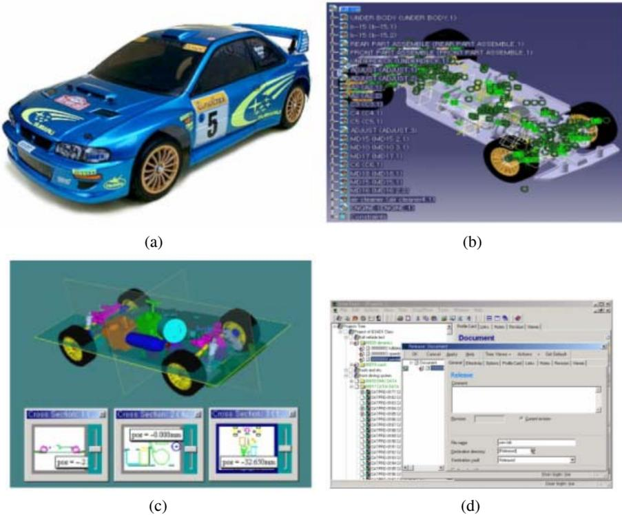
Fig. 4. Engineering design activities based on networks using various computer systems
