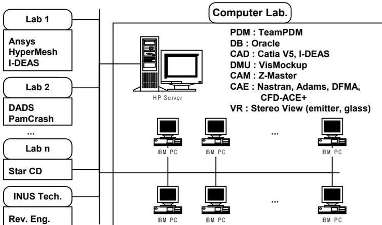
Fig. 2. System construction for network based engineering design education
